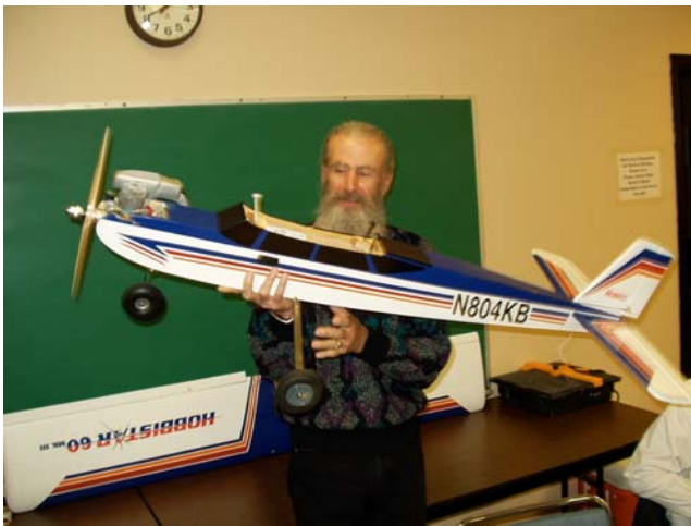
Bradford Walters – Modified Hobbistar 60 with bolt-on wings and dual servos on ailerons.
