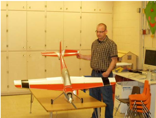
Aviv Shoval – Focus Pattern Plane 120 engine A123 batteries, 9.5 lbs.
