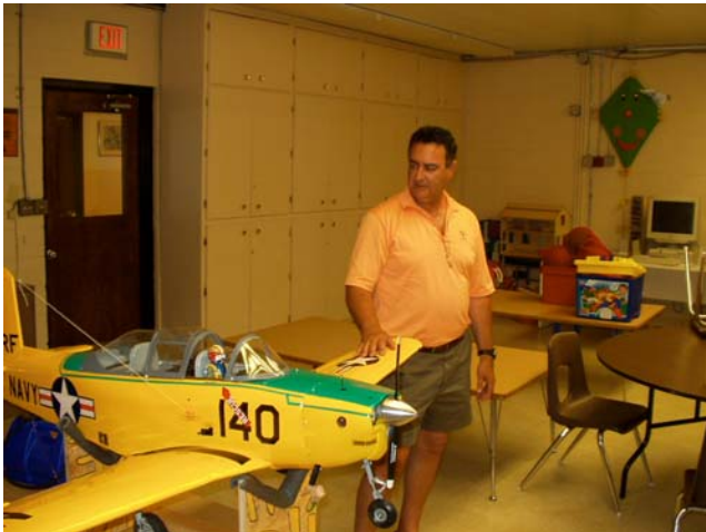
Yohay Hahamy – Top Flite T-34 Mentor, .91FX engine, A123 battery, sliding canopy, retracts, full lighting, 15.5 lbs.
