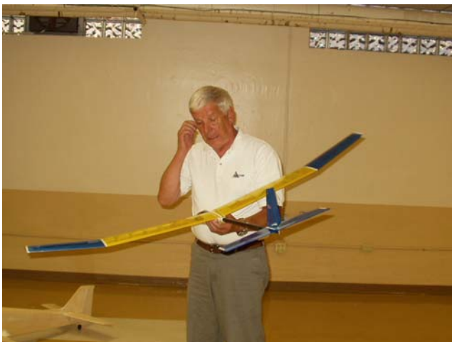
Rich Frost – Zephyr. Carbon fiber boom, fiberglass pod. If using transparent covering wait a few days after any glue use.
