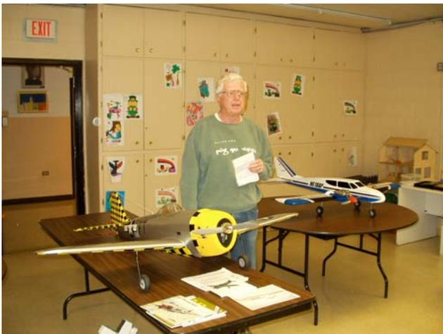
**Jim Keehan** showed a P-47 built from a Top Flight kit. He gave a bit of historical info on the plane. His kit has electric retracts from [www.lado-tech.com](http://www.lado-tech.com) and a .91 4-stroke engine.
