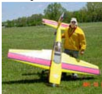
take much to get a plane together. I used 1/2 a wing from a crashed Tiger 60 and part of its tail. For a fuse I used the long ailerons that came with my Ultra Stik (I used the split ailerons on the Stik and these were going to get thrown out). You can also use PCV gutter pipe for a fuse. Basically I
