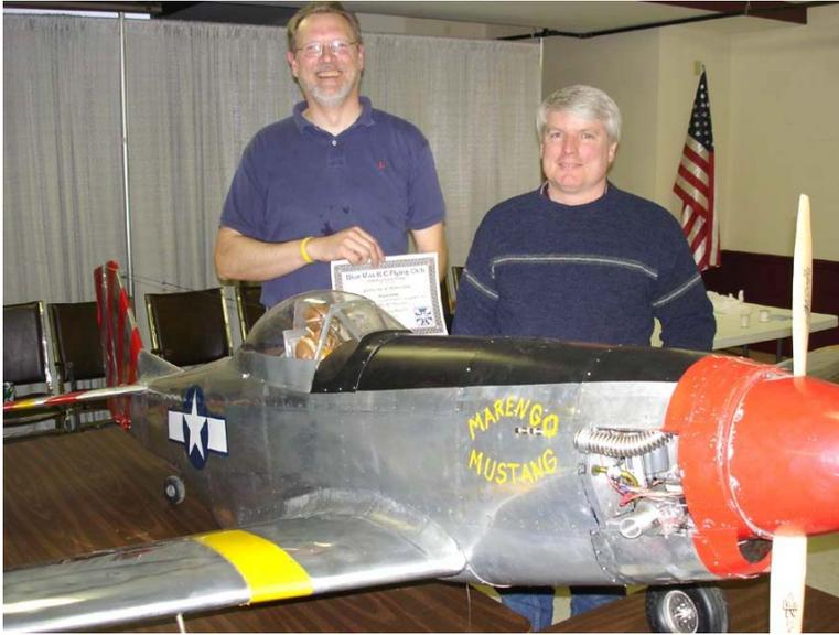
The plane is impressive – wingspan is 111“. Fuselage length is 96.5“. Wing area 14.5 Sq. feet. Wing Load 36 oz/sq ft. Dry weight of this plane is about 33 Lb. It is powered by a Zenoah G-62 gas engine. It first flew in November of 2004.
