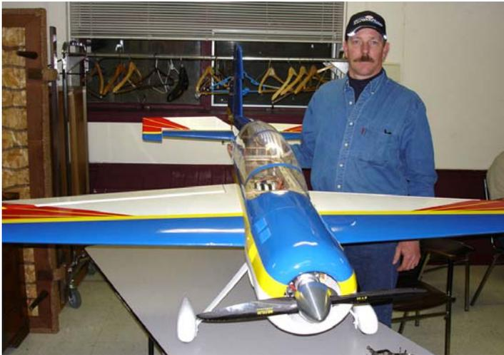
**Dennis Brumley** showed his Yak 54 from Extreme Flights. It is about a 30% sized airplane and is powered by a DA-50 gasoline engine. It weighs about 16 lb. According to Dennis this is one of the best ARF's he has ever built.
