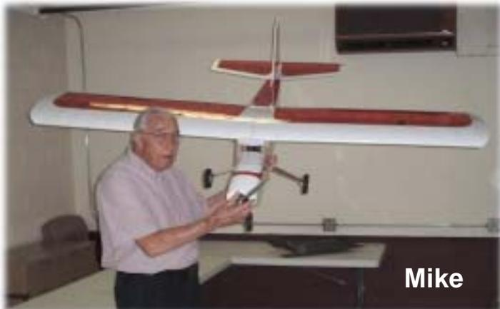
**Mike McGee** treated us to views of his new SIG Kadet Sr with an 80 inch wingspan. Mike's model is electric powered with a Model Motor AXI 4120 brushless motor. The model weighs 7.75 lbs, has 12 cells with 22 volts. It will cruise at top speed for 8 minutes. More sedate speeds increase flying time to 20-25 minutes. Eric at Venture Hobbies was credited for the plane's setup.
