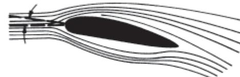
EXCESSIVE ANGLE OF ATTACK. AIR FLOW IS BROKEN. NO LIFT TO SUSTAIN THE AIRPLANE
