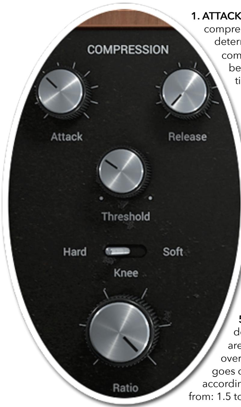
**1. ATTACK:** Control the Attack time of the compressor using this control. This control determines how quickly or slowly the compressor starts working the signal being passed through it. The Attack time ranges from .1ms to 30ms
