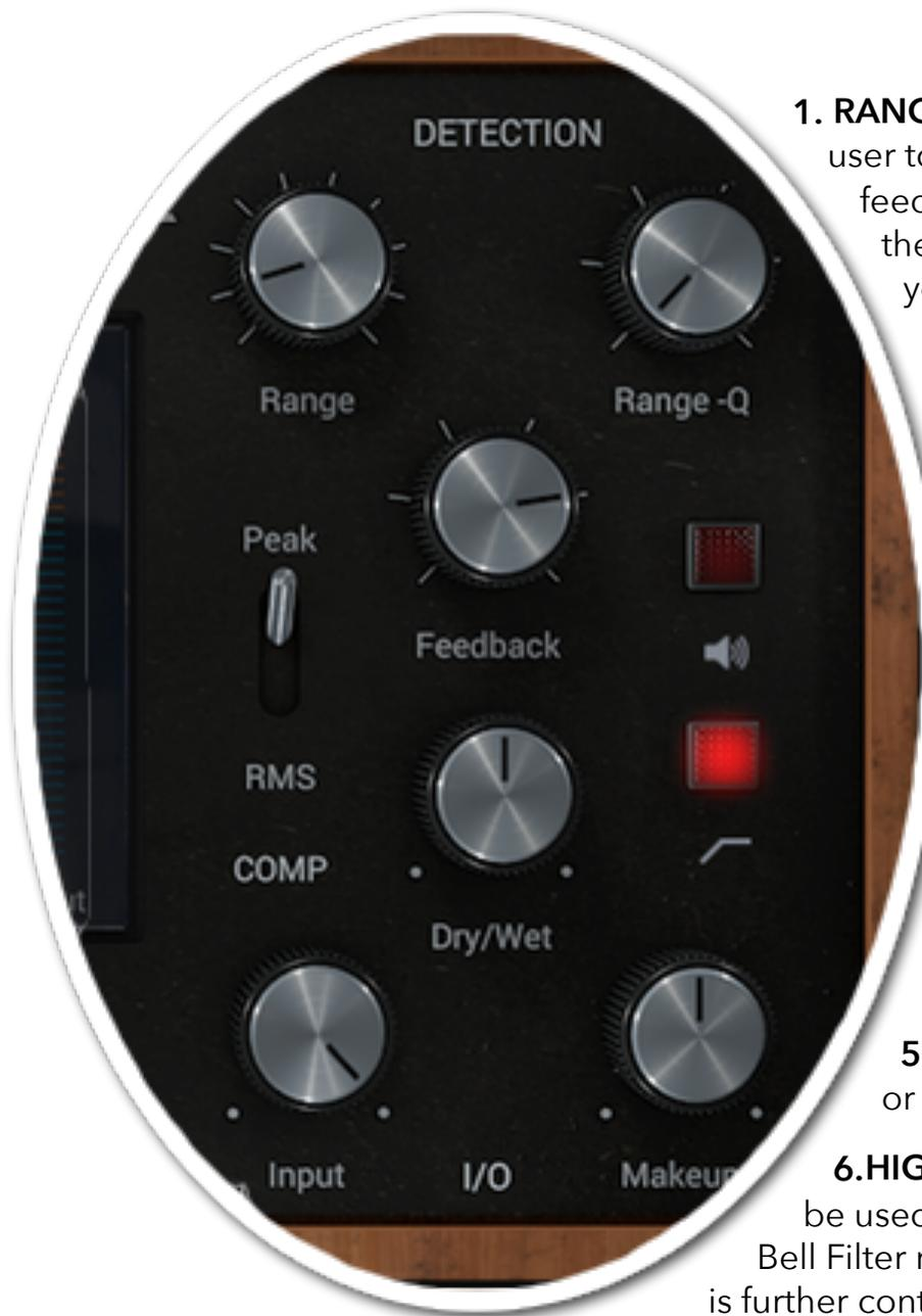
**1. RANGE (frequency):** This controls the user to select a frequency range to feedback into the sidechain circuit of the compressor. The Range Freq lets you select from 60z to 10khz
