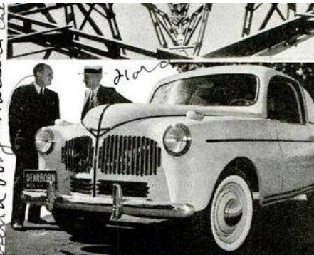
Here is the auto Henry Ford "grew from the soil." Its plastic panels, with impact strength 10 times greater than steel, were made from flax, wheat, hemp, spruce pulp
