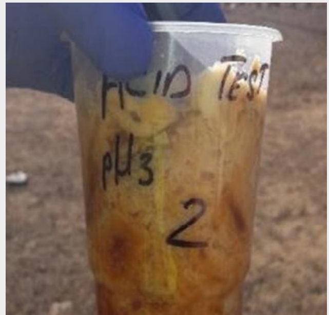
Figure 2 Field example of sodium nitrite gassed bulk emulsion decomposition caused by acidic mine water.
