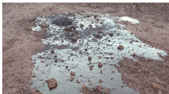
Figure 3 Mixture of decomposed emulsion and water expelled from blasthole.
