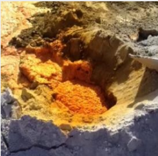
Figure 2 Field example of sodium nitrite gassed bulk emulsion decomposition caused by acidic mine water.
