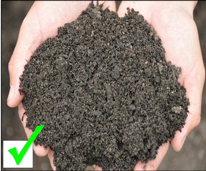
Black sand without lots of dirt. Quarry sand is also acceptable, and may be lighter in color.
