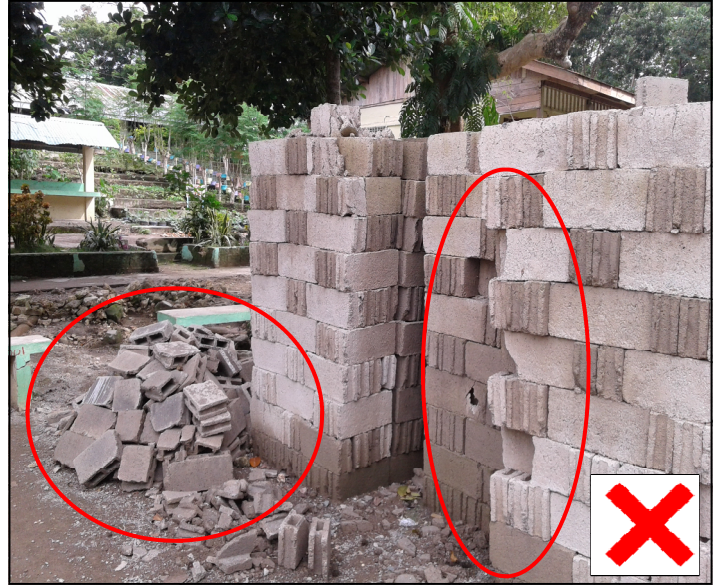
Breaks even during handling and storing.
