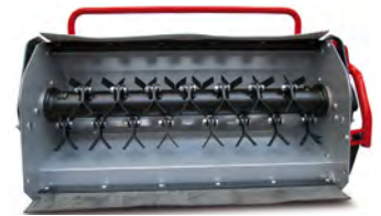
Blade view: Vertically rotating "Y" blades.
