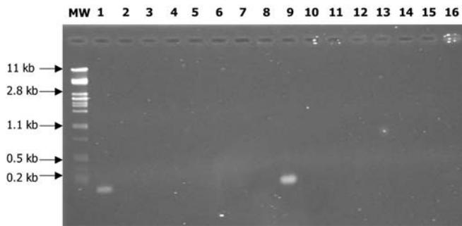
**Fig. 5** Specificity PCR analysis of two event-specific primer pairs for CBH-351 maize. Lane 1–8 event-specific primer pair nos1 NEST/SL2 tested on CBH-351 maize, non GMO maize, BtXtra maize, T25 maize, MON810 maize, GA21 maize, Bt11 maize and Bt176 maize. Lane 9–16 event-specific primer pair nos1 NEST/SL1 tested on the same DNA samples as described for the nos1NEST/SL2 primer pair
