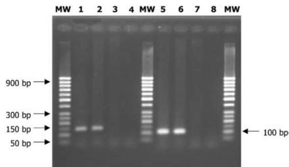
**Fig. 4** Qualitative PCR analysis of two event-specific primer pairs for CBH-351 maize. *Lane 1–4:* event-specific primer pair nos1NEST/SL1 (amplicon size 138 bp) tested on CBH-351 maize (analysis performed in duplo, lane 1 and 2), non-GMO maize (lane 3) and negative water control (lane 4). *Lane 5–8:* event-specific primer pair nos1NEST/SL2 (amplicon size: 100 bp) tested on the same DNA samples as described for the nos1NEST/SL1 primer pair. *MW* GeneRuler 50 bp DNA ladder
