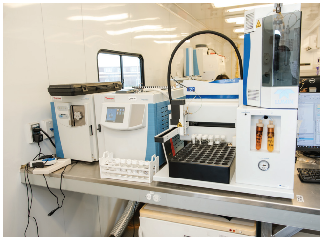
A gas chromatograph, which detects low-level organic contaminants in water samples, at the Montebello Filtration Plant.
