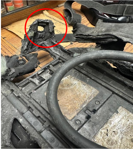
Cpt. Rinaldo’s SCBA – Shoulder Strap Failure Due to Heat (Strap and Clips)
