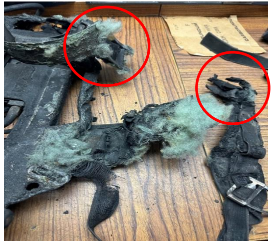
Cpt. Rinaldo’s SCBA – Failure of Cylinder Securing Strap and Shoulder Strap
