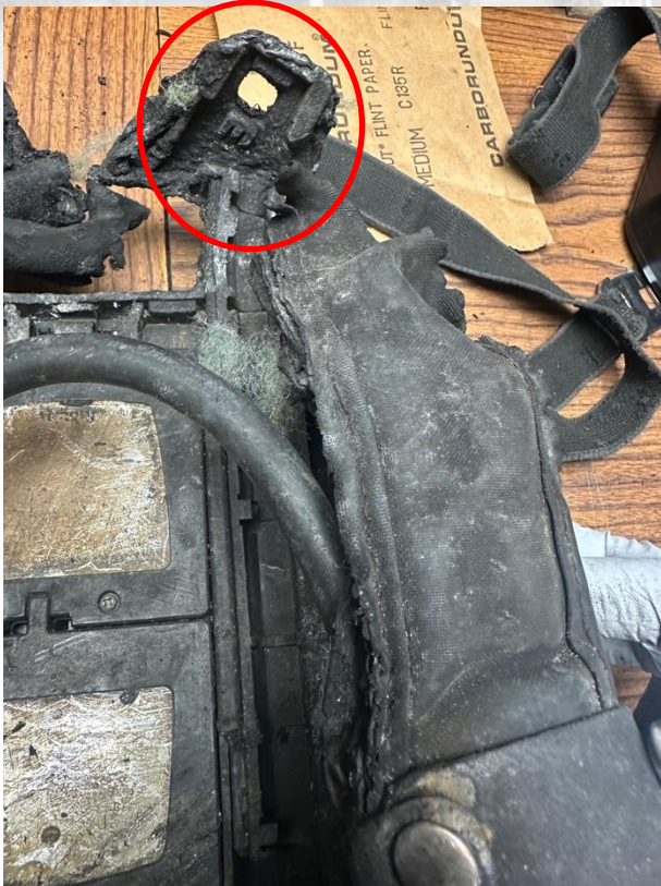
Cpt. Rinaldo's SCBA – Failure of Structural Clip Due to Heat and Elongation
