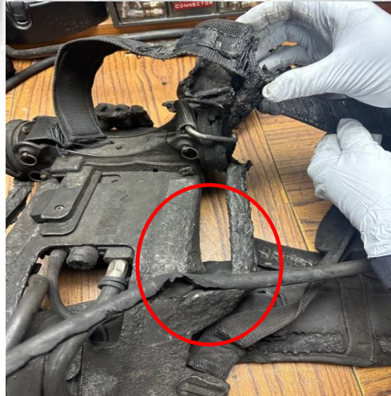
EMT/FF Pitts' SCBA – Failure of Cylinder Securing Strap
