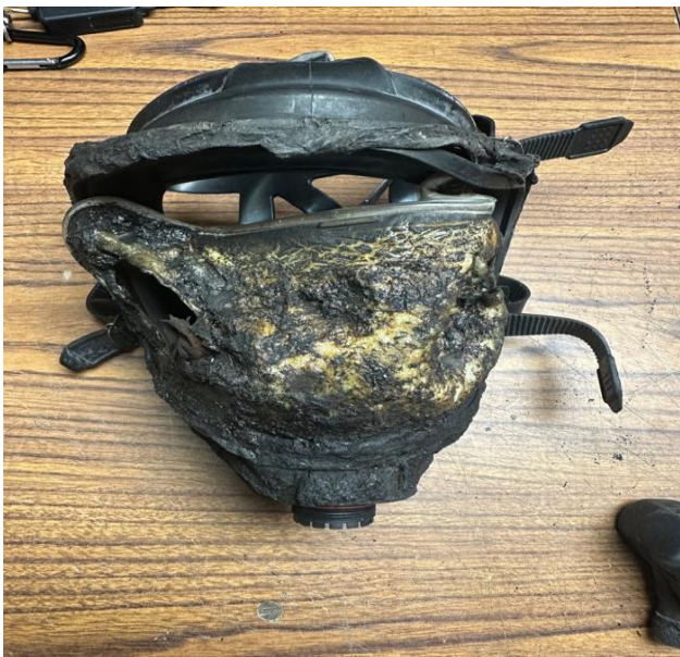
Cpt. Rinaldo's SCBA – Failure of Face Piece
