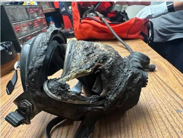
Cpt. Rinaldo's SCBA – Failure of Face Piece
