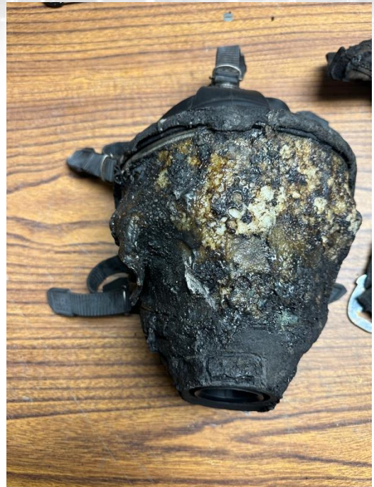
EMT/FF Pitts' – Failure of Face Piece
