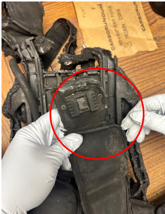
EMT/FF Pitts' SCBA – Failure of Waist Strap and Connection Points to Harness
