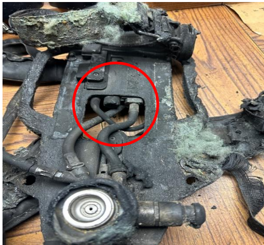
Cpt. Rinaldo’s SCBA – Beginning Stage of Failure in Lung Demand Valve Hose
