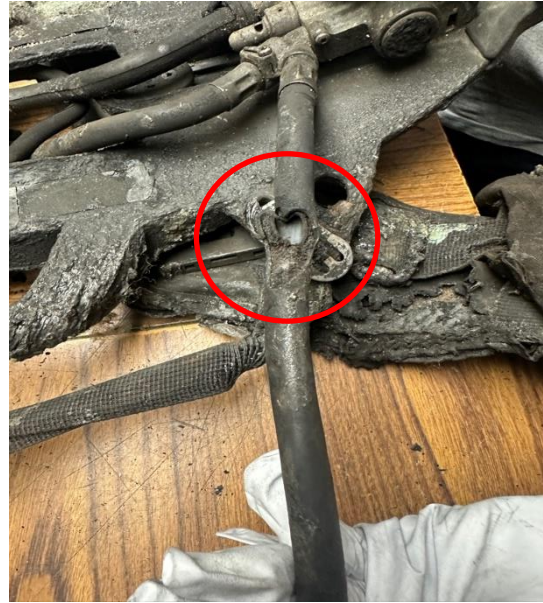
Cpt. Rinaldo’s SCBA – UEBSS Failure 3” from Regulator Block of Buddy Breather whip)
