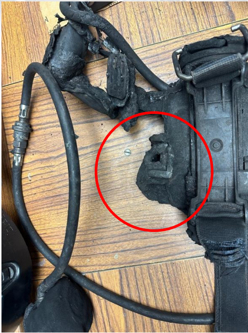
EMT/FF Pitts' SCBA – Failure of Shoulder Straps and Connection Point
