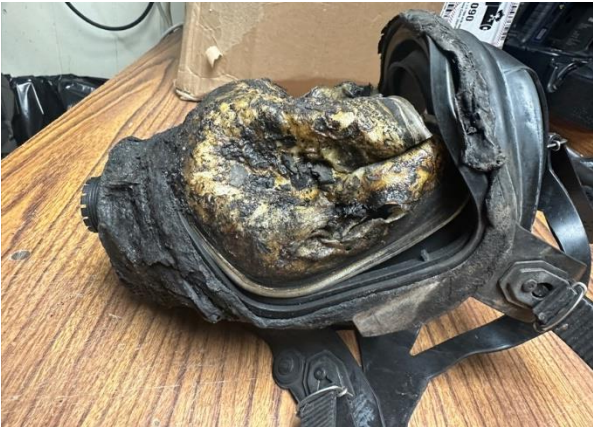
Cpt. Rinaldo's SCBA – Failure of Face Piece
