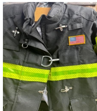
Equipment Photo #7 Turnout D-ring
