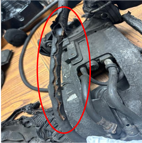
EMT/FF Pitts' SCBA – UEBSS Failure 9" from Regulator Block of Buddy Breather
