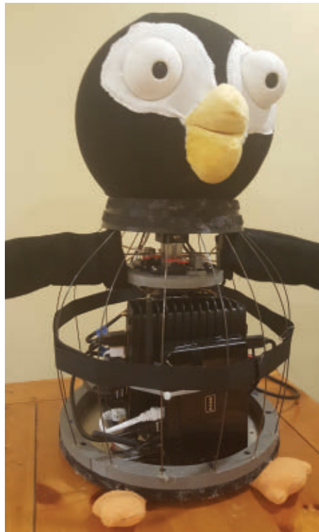
PABI’s electronic and servo insides are guarded by spring steel ribs and a plush, stuffed exterior.
