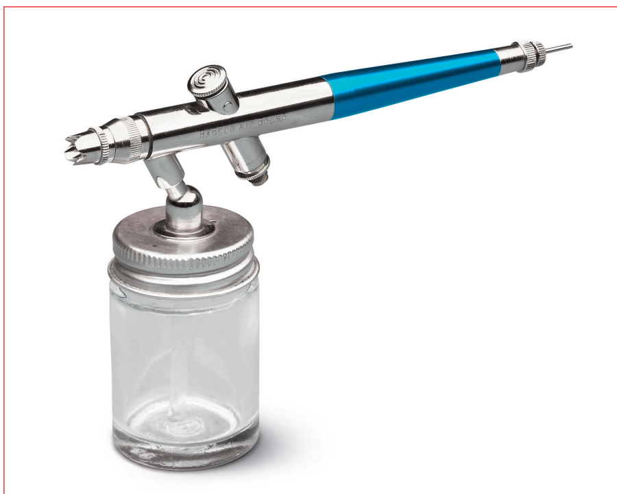
Fig. 3 The Hybrid airbrush is a single-action airbrush with internal mixing. The brush has the longitudinal needle found on double-action brushes, but the paint volume is controlled by turning the knurled knob on the end of the needle instead of with the trigger. FineScale Modeler photo
