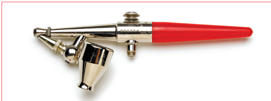
Fig. 1 Single-action airbrush. With this style of brush, the air flow draws the paint up from the color cup (or bottle) into the angled paint nozzle. The knurled nozzle adjusts paint volume, and the button on the top controls the air flow.
