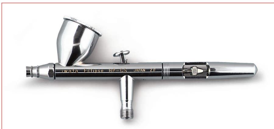
Fig. 2 Double-action airbrush. On a double-action airbrush the air flow is controlled by pushing the trigger down; the paint flow is controlled by pulling the button back. The paint flows into the body of the airbrush from a gravity-feed cup. FineScale Modeler photo
