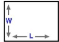
For areas that are not rectangular, break up the area into smaller rectangles (as shown in Figure 2). Multiply the width times the length for each small rectangle, then add up all results to calculate the overall square footage.
