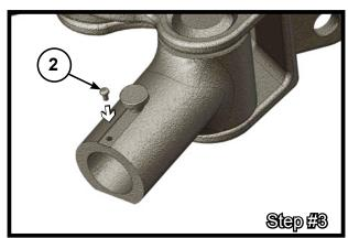
3. Install the rivet into the hole thru the locking pin springs and bar pivot of the hitch head.
