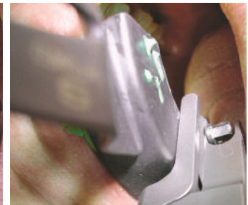
Place the jaws of the Easy X-Tractor® between the surface of the Protector and the head of the Screw.
