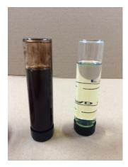
The picture on the left shows two vials of diesel fuel where sulfuric acid has been added. In the vial on the left Stanadyne Performance Formula has been added while DieselBOOST Diesel Fuel Upgrade has been added to the vial on the right.
