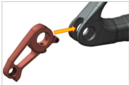
Before installing the new hanger first make sure the area is clean; insert the hanger.
