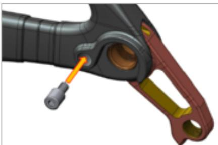
Insert the second bolt in the rear of the dropout (Max torque 1.5 N/M)
