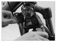
If you have disc brakes (hydraulic or mechanic), check the position of the brake pads through the inspection window. In this way you will be able to tell after the removal whether the brake pads are still in their correct position. Read the manual of the brake manufacturer on this SCOTT info CD.
