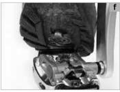
Make sure that the pedals and shoe soles are always clear of mud and other foreign bodies and grease the lock-in mechanism with lubricant at regular intervals (a).
