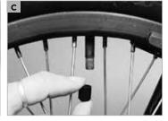
With Presta valves you first have to undo the small knurled nut a little and depress it carefully until air starts to escape. Check the nut is tightened and seated in its stem, otherwise air may slowly leak out. Do not forget to tighten the valve by hand nut after inflating.
