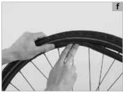
Work the tyre into the rim by approaching the valve symmetrically from both sides. Towards the end. you will have to pull the tyre vigorously downwards (a) to make the already mounted portion of the tyre slip towards the deepest part of the rim well. This will ease the job noticeably on the last centimetres.
