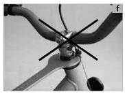
5 20 ENGLISH OWNER'S MANUAL 2017 | KIDS' TOY BICYCLE KIDS' TOY BICYCLE | OWNER'S MANUAL 2017 ENGLISH 21 | 5 Now you can move the handlebar/stem-unit up and down as a whole. Be sure not to pull out the stem too far. The mark on the stem (end. min. max. stop. limit or the like) should always remain within the tube (a). Setting the stem to a lower position can only add to your safety!
