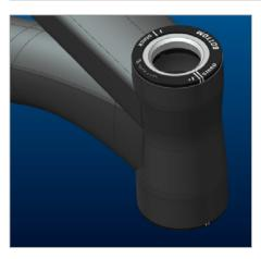
In addition Syncros Pressfit DH Adjustable headset (SCOTT part number : 228442) can be used to change the geometry (+/-1° or +/-2° head angle) and modify the ride feeling of the bike
