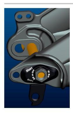
The Gambler 700 offers the possibility to change the drop out hanger in case of damage, but you also can choose between 2 different rear-axle positions which results in 2 different wheelbases.
