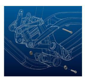
On the Gambler 700 you can adjust the BB height above ground for 10mm between its 2 positions by a geo-chip.
