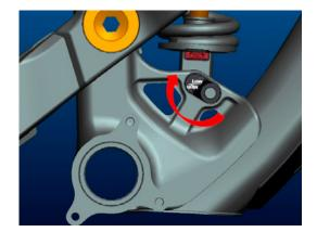
In order to change the set up please un-tighten the shockmount bolt with a 6mm allen key.
