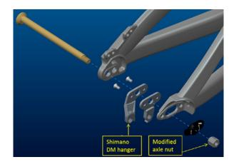
New direct mount hanger for Shimano RD in addition to old hanger for SRAM RD.
