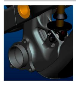
On Gambler 700 the BB standard is PF 104 with a housing width of 104mm and an inner diameter of 41mm for PressFit bearings.
