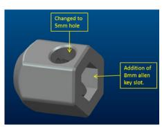
Axle nut has been modified to accept a 5mm allen key (instead of 4mm) through the nut and an 8mm allen key in the end of the nut. Still compatible with MY13.
