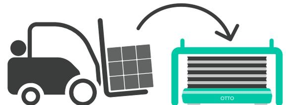
A forklift operator moves the pallet to a P&D Stand and OTTO, equipped with a lift, picks up the pallet from the stand.
