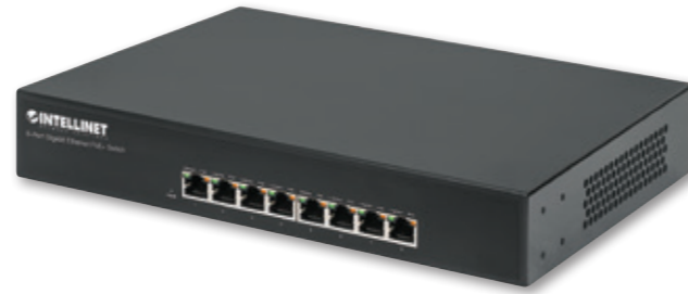
8-Port Gigabit Ethernet PoE+ Switch [560641] IEEE 802.3at/af Power over Ethernet (PoE+/PoE) Compliant, 140 W, Endspan, Desktop, 19" Rackmount
