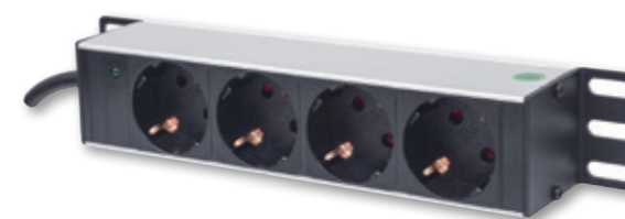
10" 1U Rackmount 4-Output Power Distribution Unit (PDU) [714020] EU CEE 7/3 Outlets, With Power Indicator, No Surge Protection, Built-in 1.8 m Power Cord with EU CEE 7/4 Plug
