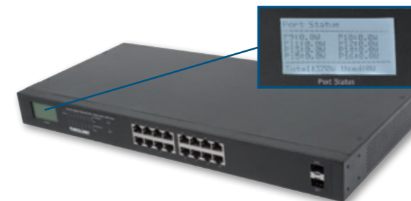
16-Port Gigabit Ethernet PoE+ Switch with 2 SFP Ports and LCD Screen [561259] LCD Display, IEEE 802.3at/af Power over Ethernet (PoE+/PoE) Compliant, 370 W, Endspan, 19" Rackmount
