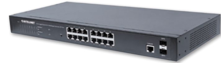
16-Port Gigabit Ethernet PoE+ L2+ Fully Managed Switch with 2 SFP Ports [561198] IEEE 802.3at/af Power over Ethernet (PoE+/PoE) Compliant, 374 W, Self-Healing Network, Endspan, 19" Rackmount
