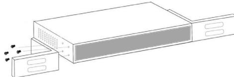
Use the screws provided with the equipment rack to mount the Intellinet data switch on the rack.
