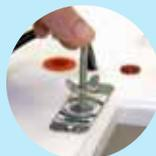
Thread adjusting screw assembly into slot until enough of shaft is visible on inside of incubator to accept wafer.
