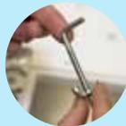
Thread wing nut onto adjusting screw.
