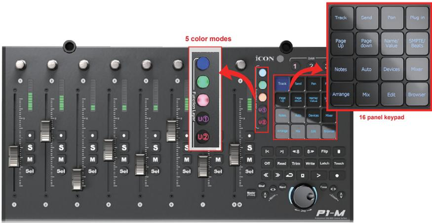
Select the DAW you would like to connect to, by selecting DAW buttons 1-3. The DAW must be set up and configured previously, (see Getting Started with the P1-M). You may change which DAWs you connect to in the iMAP, (see 'How to Allocate the DAWs to the DAW Buttons').
