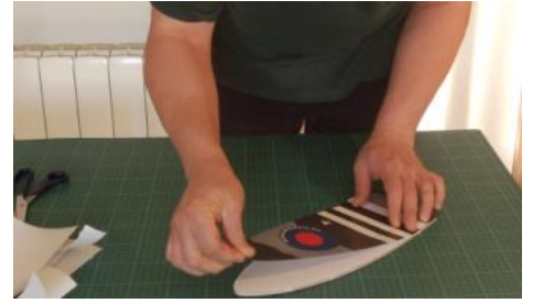
Stick the adhesive on wings, on the opposite side of the grooves
