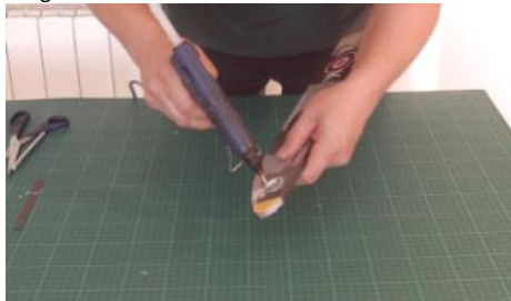
Glue the nose weight -this case a nut, approx. 52 gr.
