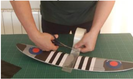
Reinforce the joint with fiberglass tape
