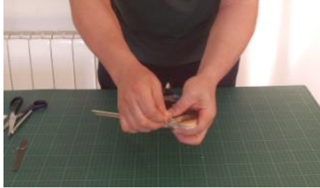
Take 2 bamboo BBQ skewers, stick them to the fuselage -1cm, tie the edges with tape, through the weight hole
