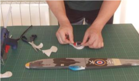
Apply the adhesives to the rudder
