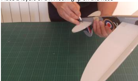
Cut two incision in the horizontal stabiliser
