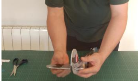
Insert the horizontal stabilizer, be sure it is centered, perpendicular, etc. and glue it
