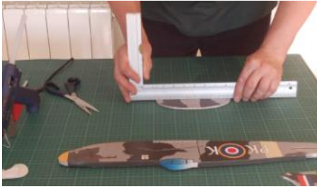
Mark the horizontal stabilizer both sides, pressing with a squad
