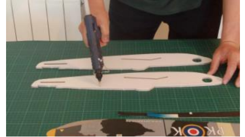
Glue the two sides of the fuselage
