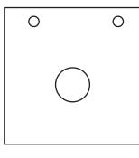
Firewall - 1/8"plywood or similar Should print at 40mmX40mm
