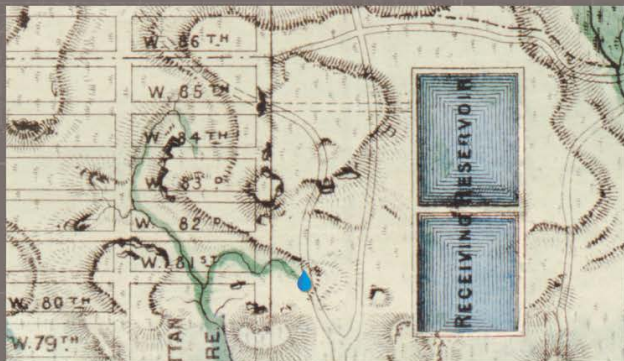
The location of Tanner's Spring is identifiable on this map from 1865. It shows the original streams and watercourses on Manhattan Island, overlaid by the street grid and park. The spring fed into a drainage system that ultimately connected all the way to the East River.
