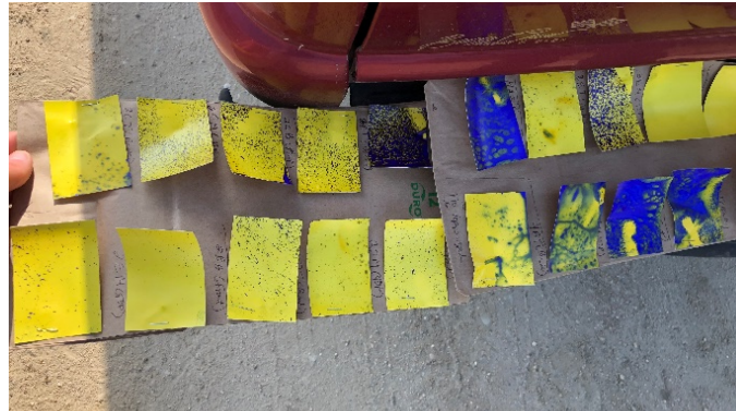
Figure 3. The smartphone app 'SnapCard' uses images from water-sensitive cards to help growers determine percent spray coverage on plants.
