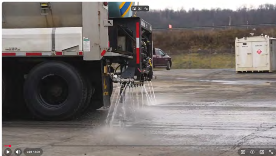
NYS DOT uses liquid salt brine to fight snow and ice during winter storms. Watch the video as Highway Maintenance Supervisor Jim DeLong explains the process.
