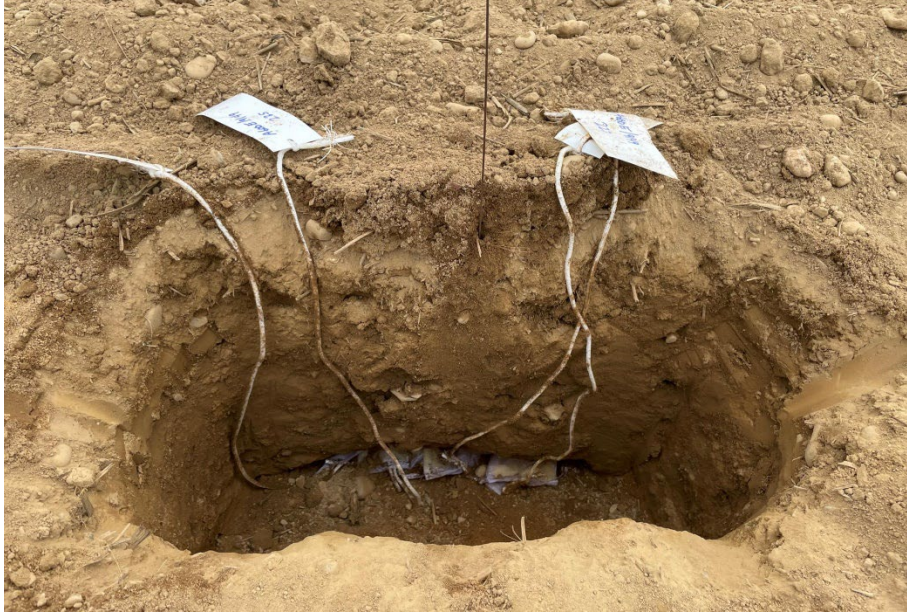
Picture of resin bags in hole in ground: resin bags are inserted 18 inches below the soil profile to capture nitrate leaching
