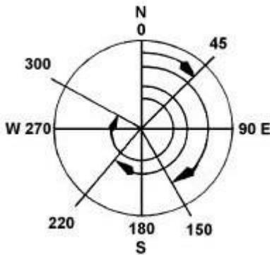
Figure 5. Azimuths are read from azimuth compass
