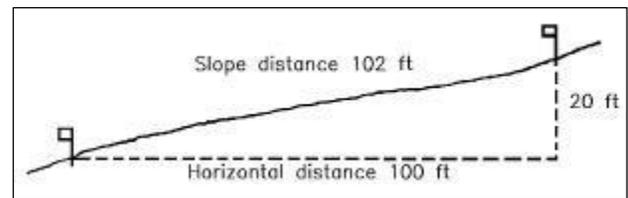
Figure 4. Estimating horizontal distance on a 20 percent slope
