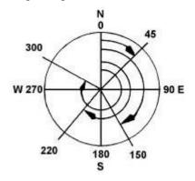
Figure 5. Azimuths are read from azimuth compass
