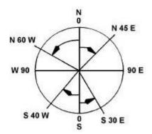
Figure 6. Bearings are read from a an quadrant compass
