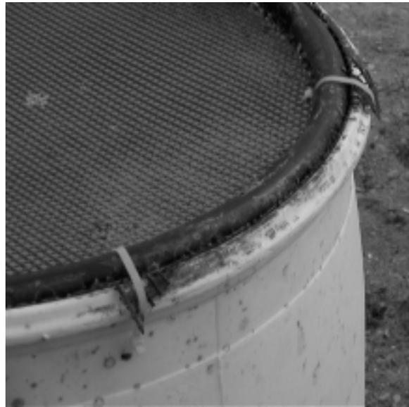
Figure 7 – Coarse mesh held on by cable ties
