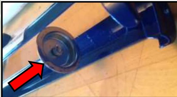
Grind down plunger head so it will fit
