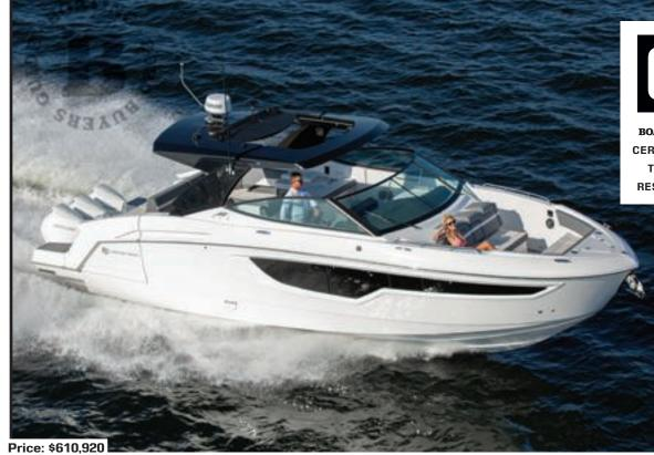
SPECS: LOA: 38' BEAM: 12'6" DRAFT (MAX): 44'3" DRY WEIGHT: 23.916 lb. SEAT/WEIGHT CAPACITY: Yacht Certified FUEL CAPACITY: 335 gal HOW WE TESTED: ENGINES: Twin 300 hp Mercury Verado DRIVE/PROPS: Outboard/16" x 18" 4-blade GEAR RATIO: 1.75:1 FUEL LOAD: 200 gal. CREW WEIGHT: 850 lb.
