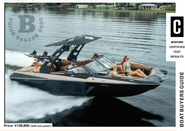
SPECS: LOA: 23'0" BEAM: 8'6" DRAFT (MAX): 2'8" DRY WEIGHT: 5,400 lb. BALLAST: 4,670 lb. SEAT/WEIGHT CAPACITY: 16/2,256 lb. FUEL CAPACITY: 58 gal. HOW WE TESTED: ENGINE: Malibu Monsoon M5 Di DRIVE/PROPS: V-Drive/Acme 3077 17" x 15" 4-blade Nibral GEAR RATIO: 2.0:1 FUEL LOAD: 45 gal. CREW WEIGHT: 360 lb.
