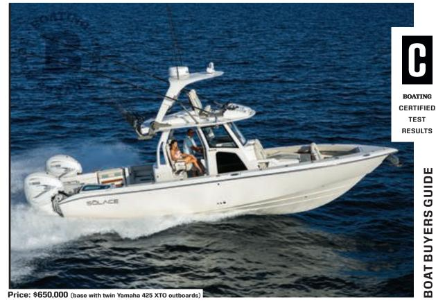
SPECS: LOA: 38'0" BEAM: 10'6" DRAFT (MAX): 1'10" DRY WEIGHT: 12.000 lb. (with power) SEAT/WEIGHT CAPACITY: Yacht Certified FUEL CAPACITY: 323 gal HOW WE TESTED: ENGINES: Twin 425 hp Yamaha 425XTO DRIVE/PROPS: Outboard/Yamaha XTO OS 16% x 20" 3-blade stainless steel GEAR RATIO: 2.037:1 FUEL LOAD: 125 gal. CREW WEIGHT: 1,000 lb.
