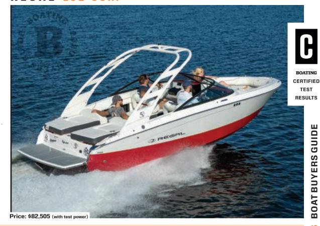
SPECS: LOA: 22'4" BEAM: 8'6" DRAFT (MAX): 2'10" DRY WEIGHT: 3,900 lb. SEAT/WEIGHT CAPACITY: 12/1,640 lb. FUEL CAPACITY: 56 gal.
