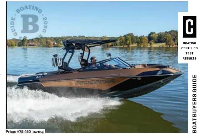
SPECS: LOA: 21'5" BEAM: 8'6" DRAFT: 2'3.5" BALLAST: 3,700 lb. DRY WEIGHT: 4,500 lb. SEAT/WEIGHT CAPACITY: 15/2,100 lb. FUEL CAPACITY: 45 gal. HOW WE TESTED: ENGINE: 350 hp Indmar Raptor DRIVE/PROP: V-drive/OJ 15.5" x 16.5" GEAR RATIO: 1.76:1 FUEL LOAD: 41 gal. CREW WEIGHT: 310 lb.
