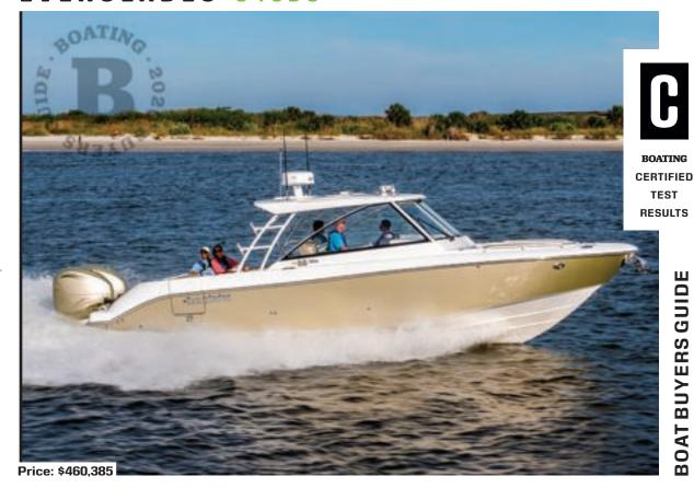
SPECS: LOA: 33'6" BEAM: 11'11" DRAFT: 2'81/4" (drives up) DRY WEIGHT: 13,000 lb. SEAT/WEIGHT CAPACITY: Yacht Certified FUEL CAPACITY: 300 gal. HOW WE TESTED: ENGINES: Twin 425 hp Yamaha XTO DRIVE/PROPS: Outboard/16 %" x 19" 3-blade stainless steel GEAR RATIO: 1.79:1 FUEL LOAD: 148 gal. CREW WEIGHT: 600 lb
