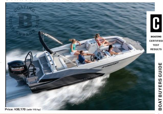
SPECS: LOA: 20'11" BEAM: 8'6" DRAFT (MAX): 2'11" DRY WEIGHT: 2,685 lb. SEAT/WEIGHT CAPACITY: 14/1,900 lb. FUEL CAPACITY: 45 gal.
