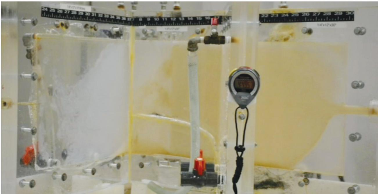
The slot flow testing showed excellent proppant transport with no settling. (Source: BJ Services)
