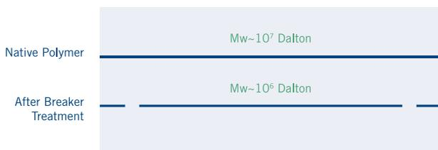
Randomly broken polymer fragments Mw in this range could likely cause more significant formation damage
