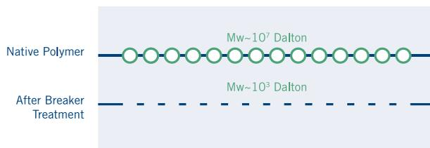
Orderly broken polymer fragments Mw in this range leaves no formation damage
