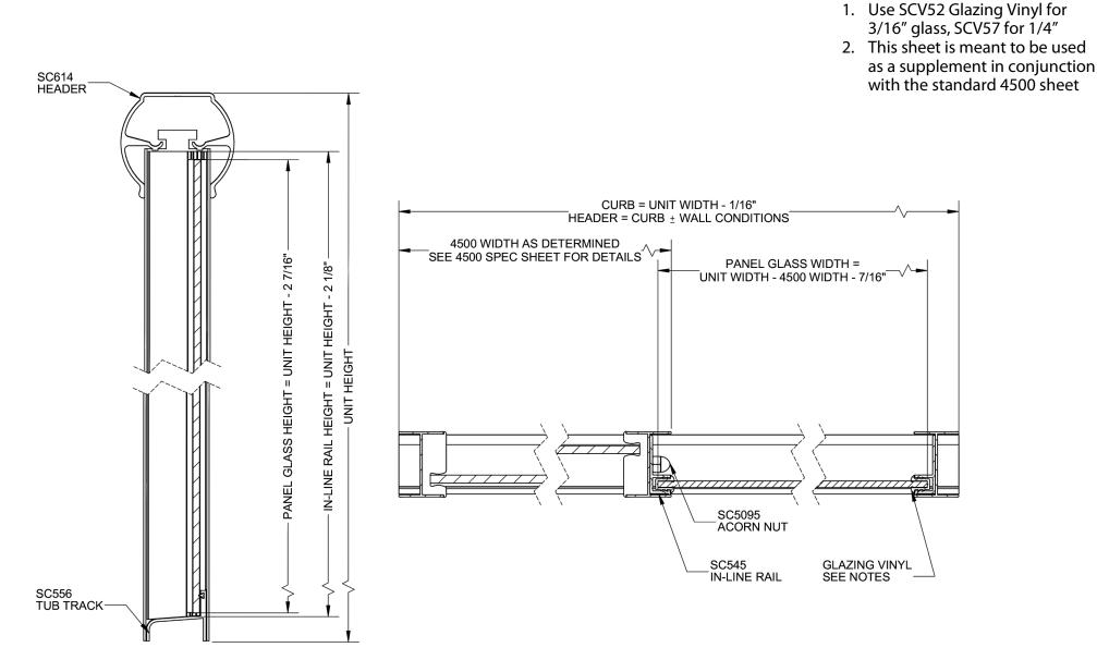
NOTE: GLAZING MATERIAL FOR ALL KD UNITS AND GLAZED UNITS MUST CONFORM TO ANSI Z97.1 AND CPSC STANDARD 16 CFC 1201 CATEGORY 1 & 2
