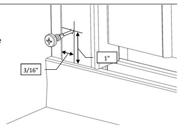
14 Install the Latch to the Door Panel by placing the Latch Vinyl on the glass first, then pressing the latch over top of the Vinyl. Be sure to install the Latch directly in the middle of the two holes in the Door Panel. Carefully cut any excess vinyl not covered by the Latch.
