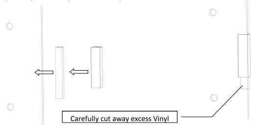
**15** Close the **Door** into the **Strike Vinyl** and gently mark on the **Strike Jamb** where it meets the bottom of the **Latch**. Remove the **Strike Vinyl** and take out the smaller insert of the **Vinyl**. Cut the insert at the marked height. Then cut 3" off of the top portion of the **Insert**.
