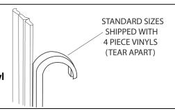
**11** Once the **Glass Panel** is set in place, cut two pieces of the **Vinyl** 1/2" longer than the exposed opening. Cut both ends of each **Vinyl** square so it will sit tight against the side of the **Wall Jamb**.
