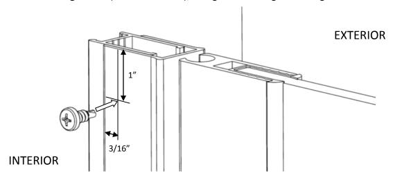
16 After the top Screw is in place, install another Self Drilling Screw into the bottom of the Hinge Jamb and Wall Jamb 1" above the Curb and 3/16" from the edge of the open side of the Hinge Jamb (see illustrations), being sure it also goes through the Wall Jamb.
