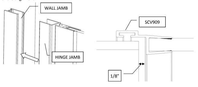
**15** Once the **Vinyls** are aligned and the **Hinge Jamb** is over the **Wall Jamb**, inside the shower insert one of the **Self Drilling Screws** into the **Hinge Jamb** about 1" from the top and about 3/16" from the edge of the open side of the **Hinge Jamb** (see illustrations), being sure it also goes through the **Wall Jamb**.
