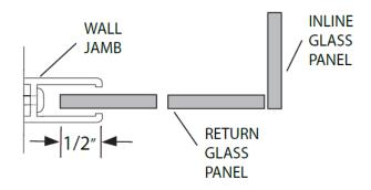
**NOTE**: Depending on any out of plumb or level conditions, the panel/metal overlap might vary from 1/4" to 3/4". Use a level to determine if this is necessary.
