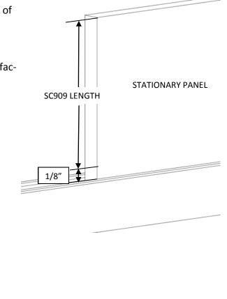
14 With a helper inside, slide the Hinge Jamb over the Wall Jamb, the flush side of the Hinge Jamb and Hinge Rail will be at the top. While keeping the Hinge Jamb over the Wall Jamb, align the Door Panel and Vinyl so there is a continuous 1/8" gap. TIP: Put an 1/8" Setting Block between the Door Panel and Vinyl to help with the alignment.
