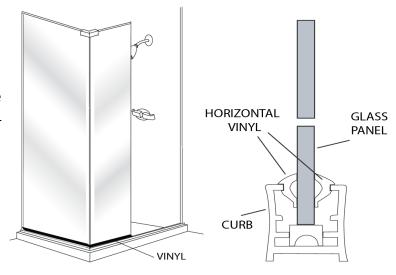
**12** Measure the distance from the top of the **Curb** to the top of the **Glass Panel** and subtract 1/8". Cut the **SC909 Vinyl** to this length.
