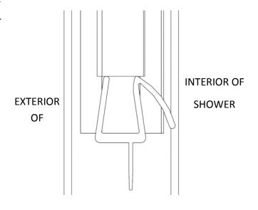
**20** Install the **Drip Vinyl** so it is flush against the **Glazing Vinyl** on the **Hinge Rail**. Close the door until it rests against the **Glass Panel/SCV909 Vinyl**. Notice where the **Drip Vinyl** lines up with the **SCV909 Vinyl** and cut the **Drip Vinyl** flush (Illustration Below).
