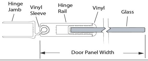
**10** The glazing **Vinyl** for this door are designed to fit tightly between the glass and metal frame.
