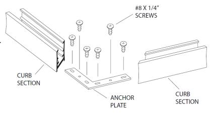
**4** Draw and measure the centerline of the threshold. Once the measurement is made cut the **Curb** sections accordingly so they will sit on this centerline. These cuts may have been already performed by the factory.
