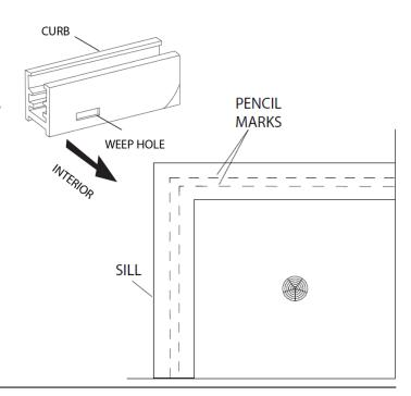
**5** Place one **Wall Jamb** into the **Curb** against the wall. Using a level, plumb the **Wall Jamb** and mark the hole locations on the wall with a pencil. Repeat this step for the other **Wall Jamb**. Remove all parts and drill the holes.
