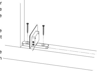
With both hinges open and aligned to each other, use a suction cup to carefully move the Door Glass into the opening over the hinges.
