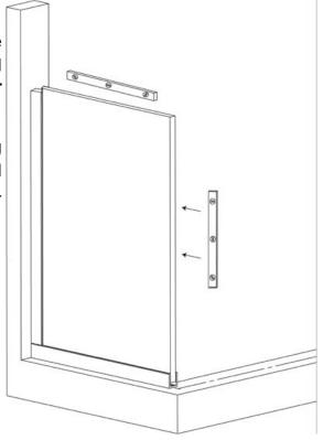
With the two Header pieces laying on a flat surface with the top of the Header facing upward, slide the 90° Header Bracket into one half of the Header and tighten the set screws.
