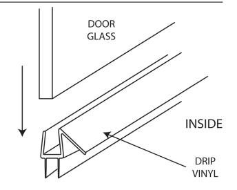
On the interior face of the glass, place a strip of low tack tape on the glass about 1/8" to 3/16" away from edge of the u-channel both vertically and horizontally. Run a small bead of silicone along this edge. Next, on the interior, run a bead of silicone between the u-channel and the threshold and also between the u-channel and the wall. After completing, remove the tape before silicone sets.
