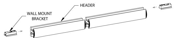
NOTE: Your header may differ in external shape than what's shown. However, internal geometry and installation procedures are the same.
