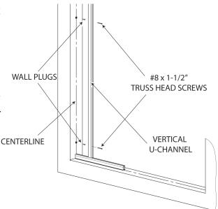
Insert a small amount of silicon into each drilled hole, then insert a wall anchor into each hole. (Note: Drill hole, then insert a wall anchor.) This must be done just before u-channel installation.
