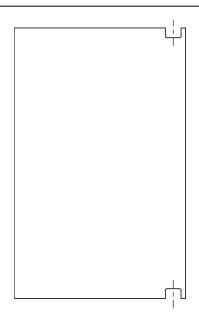
Place two 7/16" shims on the curb or threshold. These shims must remain in place throughout the installation process.
