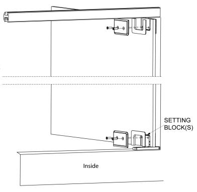
Tighten the screws, alternating so the pressure is evenly applied to the inside cover plate as you tighten the screws. Continue tightening until the screws begin to squeak.
