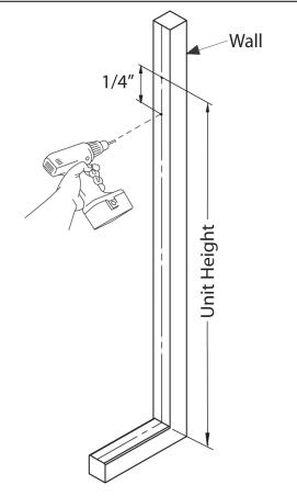
Install the Header using a Truss Head Screw on each end.
