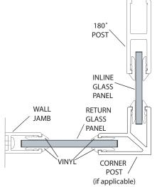
17 Cut the horizontal vinyl [S] 1/2" longer than the horizontal opening for both glass panels. Cut both ends of each piece of vinyl with a back mitre. (see illustration) This will allow them to sit tight against the face of the vertical vinyl.
