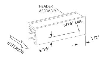
Press the header assembly over the wall jambs, 180° post and corner post, if applicable. Check both sides of the corner post for plumb. Adjust as required by varying the overlap of the header over the wall jambs. Also, plumb the 180° post, making sure to maintain the proper coverage over the inline glass panel of 1/4" to 3/4" as described in Step # 5. Mark its' location on the header and curb with a light pencil mark or a piece of tape.
