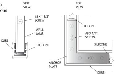
Place four setting blocks [G] into the curb, flat side up, to support the stationary glass panels (two blocks per panel). Position the blocks so they are centered about 3" from each corner of the glass panels. Set the return glass panel [H] in the curb on the setting blocks and slide into the wall jamb approximately 1/2". A piece of tape positioned 1/2" from the vertical edge will help placement.
