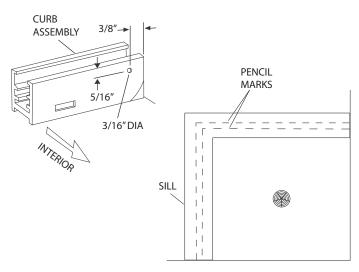
Place one wall jamb [D] into the curb against the wall. Using a level, plumb the wall jamb and mark the hole locations on the wall with a pencil. Repeat this step for the other wall jamb. Remove all parts and drill the holes. **TIP:** Tape can be used to temporarily hold the curb in place.
